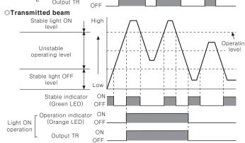
\*The waveform of "Operation indicator" and "Output TR" is for Light ON mode, it is operated conversely for Dark ON mode
