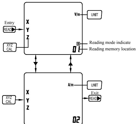
1. Press **READ** key, the display shows “**R**”(reading mode).
