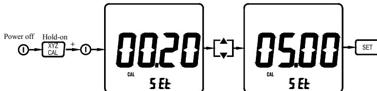
When the meter is normally turned on, the calibration factor set value will display for 2 seconds.
