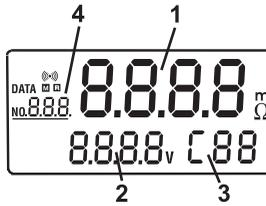
1. Measured resistance reading (or High/Low resistance limit when setting up the comparator)
