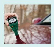
Extech's CG304 offers a non-destructive way of measuring the thickness of ferrous and non-ferrous substrates with auto recognition of the material being measured. Unique Bluetooth® interface feature wirelessly transmits measurement data to your PC for further analysis and to generate a documented report.
