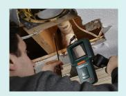
Light weight VideoScope includes a wired handset and 6mm diameter camera with 240° articulating tip for best viewing angle. Easy one-hand operation of the articulating camera tip facilitates viewing in obstructed areas where standard camera tips cannot access. Images and videos are viewed on the large high resolution color display or external monitors and can be stored in SD memory card (included) or a USB flash drive.
