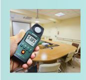
Extech's pocket-sized autoranging Light Meter offers wide light intensity ranges measuring up to 40,000Fc (400,000Lux) with high resolution to 0.01Fc (0.1Lux). Ideal for indoor lighting tests and for checking security and safety illumination in parking garages, night time ATM areas, stairwells, landings, and hallways.
