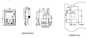
The keypad can be externally installed on an optional bracket.
