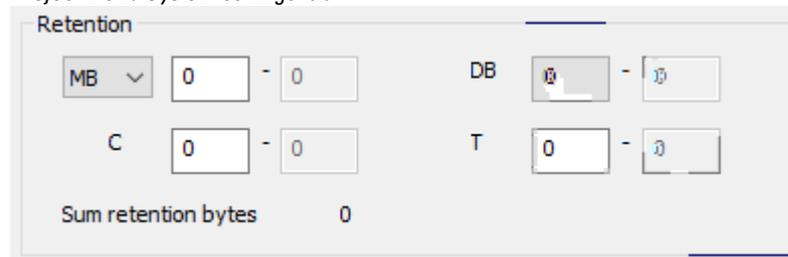
Figure 245: Screenshot of Retention section that can be found in the System settings tab in the Project view (including sample values)
