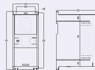
Wall mounting of 0.75-2.2kW VFDs
