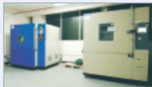
Low Pressure Test Chamber & Constant temperature and humidity test chamber
