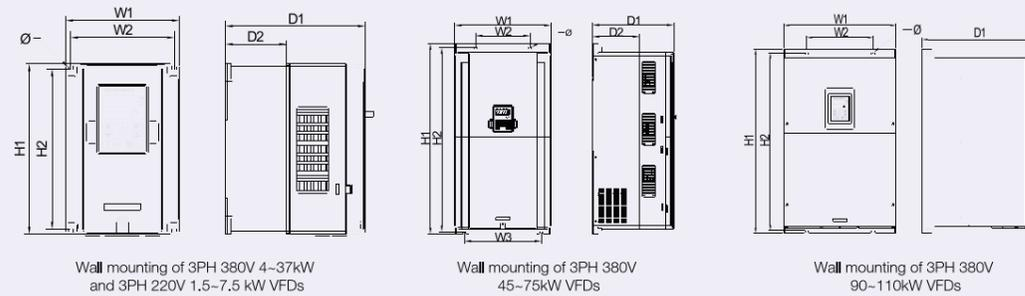
Wall mounting of 3PH 380V 4-37kW and 3PH 220V 1.5-7.5 kW VFDs
