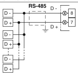
Interface type: Isolated (50 V) RS-485; Voltage levels: According to EIA standard;
