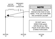
Figure 9. Single Phase Motor Connections
