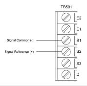
Figure 13. Analog Input Signal Connections
