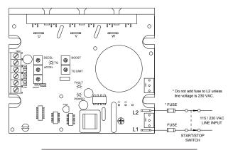
Figure 6. VFD100 and VFD300 AC Line Connections
