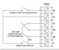
Figure 12. Potentiometer and Switch Connections
