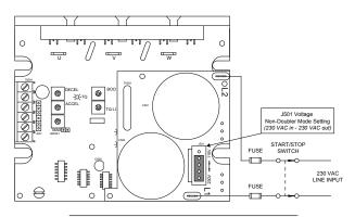
Figure 8. VFD600 Connections for a 230 VAC Line
