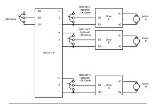
Figure 23. Single Speed Potentiometer Control of Multiple Drives
