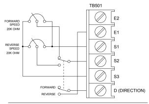
Figure 19. Independent Adjustable Speeds with a Direction Switch
