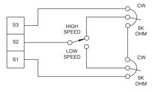
Figure 17. Adjustable Speeds Using Potentiometers In Series
