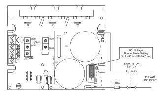
Figure 7. VFD600 Connections for a 115 VAC Line
