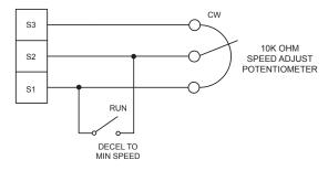
Figure 15. Run/Decelerate to Minimum Speed Switch
