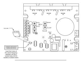
Figure 26. Carrier Frequency Capacitor Location
