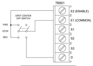
Figure 24. Quick Reversing Circuit Wiring
