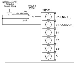
Figure 20. RUN/JOG Switch - Connection to Speed Adjust Potentiometer
