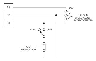
Figure 21. RUN/JOG Switch - Connection to Speed Adjust Potentiometer
