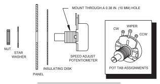
Figure 5. Speed Adjust Potentiometer
