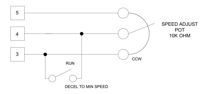
Figure 8. Run/Decelerate to Minimum Speed Switch
