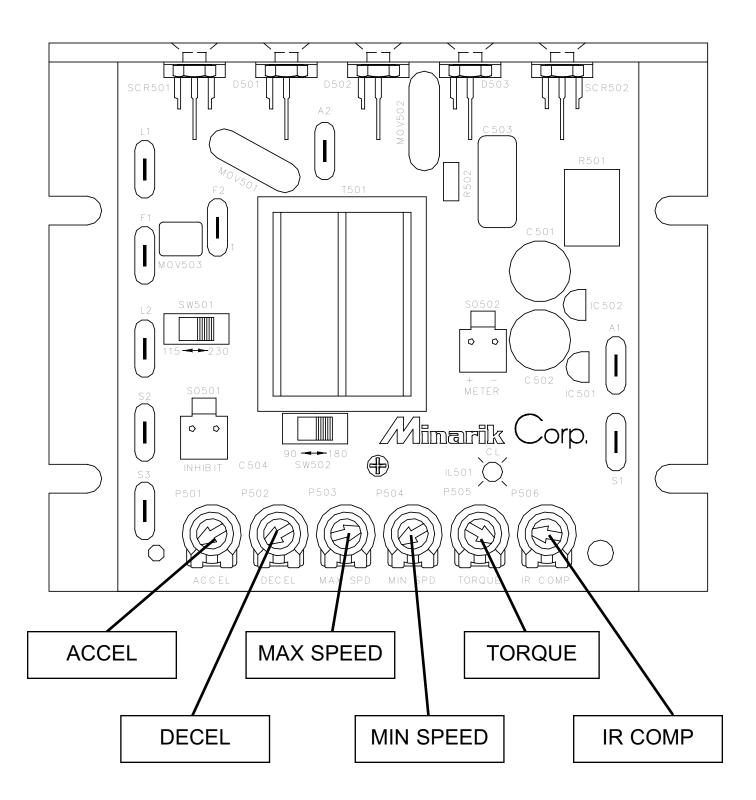
Figure 10. Calibration Trimpot Layout
