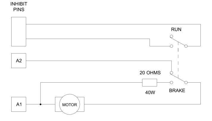
Figure 9. Dynamic Brake Connections
