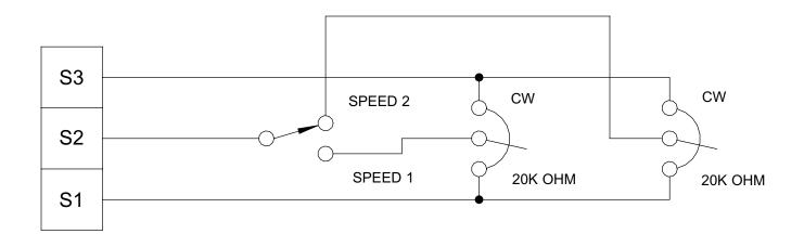
Figure 14. Independent Adjustable Speeds
