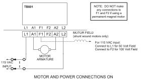
MOTOR AND POWER CONNECTIONS ON BOTTOM "POWER CIRCUIT" BOARD
