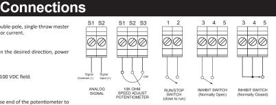
SIGNAL CONNECTIONS ON TOP "LOGIC" BOARD
