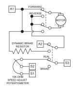
Two DPDT Switches for Independent Run/Brake & Forward/Reverse Switches
