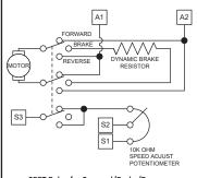
3P3T Relay for Forward/Brake/Reverse
