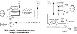
Two DPDT Switches for Independent Run/Brake & Forward/Reverse Switches In Signal Mode Operation
