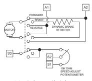
3P3T Relay for Forward/Brake/Reverse In Manul Mode operation
