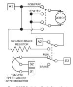
Two DPDT Switches for Independent Run/Brake & Forward/Reverse Switches In Manual Mode Operation
