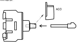
4. Turn the switch to OFF-position (0). Push the switch in place until the snap-on grips are firmly clipped on both sides of the switch.
