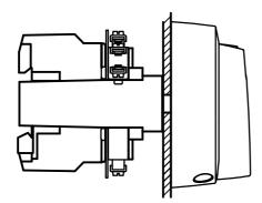
WARNING: Auxiliary contact may be broken if pushed on switch in ON-position (1).
