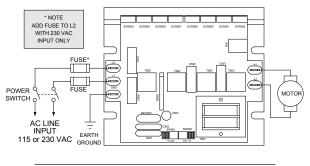
Figure 7. Power and Motor Connections (bottom board)
