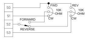
Figure 24. Independent Adjustable Forward and Reverse Speeds
