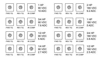
Figure 16. Recommended FWD TQ, REV TQ, and IR COMP Settings (actual settings may vary with each application)
