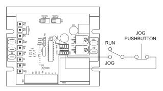
Figure 26. RUN/JOG Switch - Inhibit Connection
