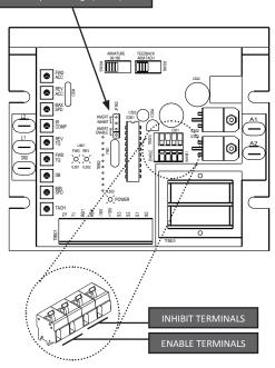
Figure 15. Inhibit / Enable Locations
