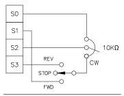
Figure 19. Forward-Stop-Reverse Switch
