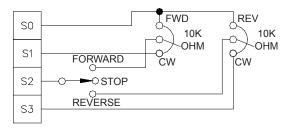
Figure 25. Independent Adjustable Forward and Reverse Speeds with Stop
