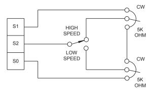
Figure 22. Adjustable Speeds Using Potentiometers In Series
