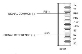
Figure 9. Analog Input Signal Connections
