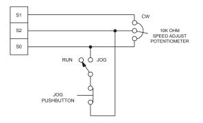
Figure 27. RUN/JOG Switch - Speed Adjust Potentiometer Connection
