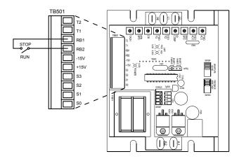
Figure 12. Regenerative Brake Switch
