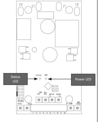
Minimum Speed (MIN SPEED): The MIN SPEED setting determines the minimum motor speed when the speed adjust potentiometer is set for minimum speed. It is factory set for zero speed. To calibrate the MIN SPEED in Unidirectional Mode:
