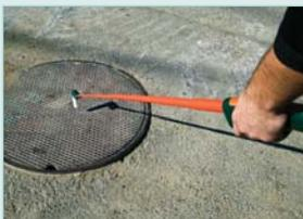
Detecting live AC Voltage on manholes with convenient telescoping probe. When Voltage is detected, audible beeper will sound and the red LED will flash on the probe tip.
