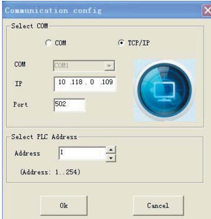
When it is correctly linked, this interface disappears automatically, and you can enter into the main interface of APB Soft. If it fails to connect, the following information will be given. And you should check if the IP address and port number are written accurately; if the cable connection is reliable and the power linkage is proper.
