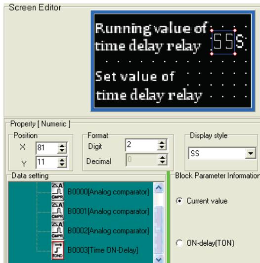
Choose the component “ **BE** ” , and select “ Function block B0003 (on-delay).The “ ON-delay ” is chosen as the parameter. Displayed digits: 2; decimal digits: 0.
