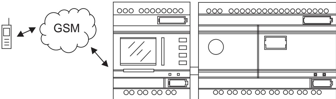
When SMS works in mode 0 APB PLC input state can be inquired and output state. time and count parameter. analog parameter can be inquired and set by sending the mobile phone instruction. The alarm message can be sent to user mobile phone by programming SMS function block in APB software.
