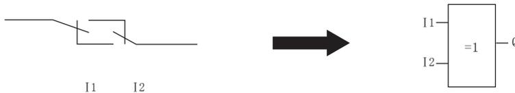
When the status of inputs is different, the output status of XOR is 1.
