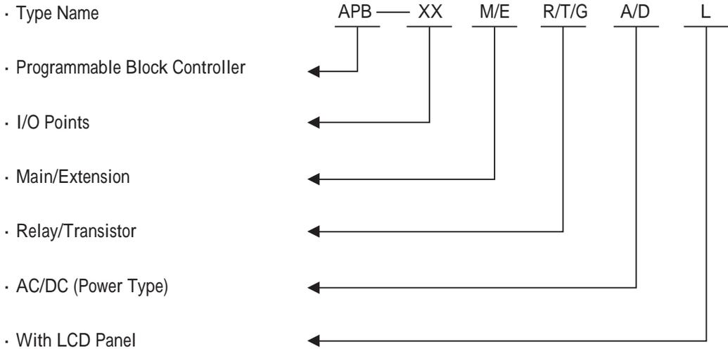
Note: M means main machine, E means extension module; R means relay output, T means NPN transistor output, G means PNP transistor output; A means AC type, D means DC type; C means real - time clock; The economical type is supplied without LCD panel, and the basic type is supplied with LCD panel.
