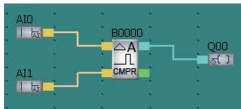
Input 1 is connected to AI0
