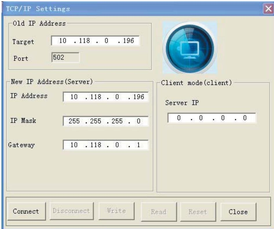
Click “ Connect ” button. If it fails to make a connection, please check the network cable. And you can restore the factory settings of the network module to link again.
