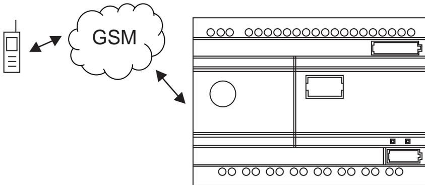
When SMS works in mode 0.Input signal SI1 has message alarming function. When the high level triggers SI1, the message “ I1ON ” will be sent to the target number to alarm。 The input and output state can be inquired and SQ1 can be set by sending the mobile phone instruction。 Input signal SI0 controls the output SQ0 directly. The SQ0 delay ON OFF time can be set by GSMMODULE software.
