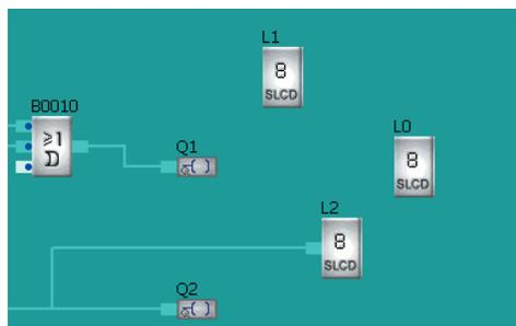
The function block L0 displays the set value and the running value of time delay relay.
