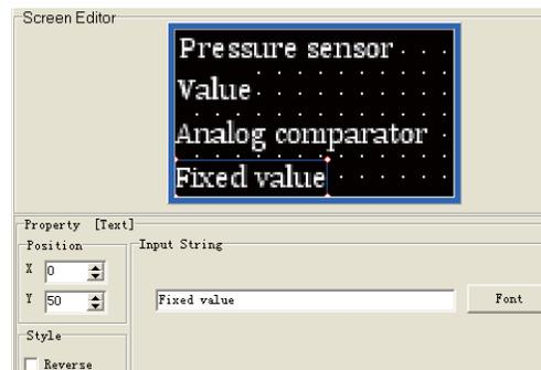
Choose the component “ **B** ” , and select “ Function block B0000 (universal analog comparator).The “ Running value of the block ” is chosen as the parameter. Displayed digits: 3; decimal digits: 2.
