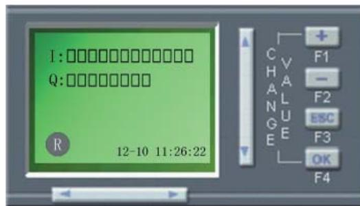
On this interface, it is able to observe PLC I/O status, and in the meantime, the current system time and PLC running status are displayed. Press “ ↑ ↓ ” key to jump to self-defined interface.
