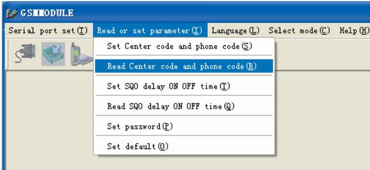
Click “ Read Center Code ” input correct password to read SMS center number from SMS module.
