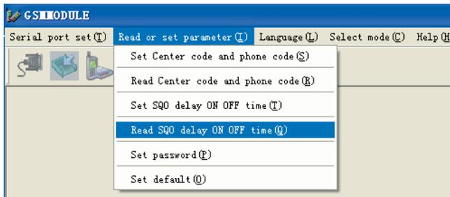
Input SQ0 Delay ON time Click “ Read SQ0 delay ON time ” and input correct password to download Delay ON time to SMS module.
