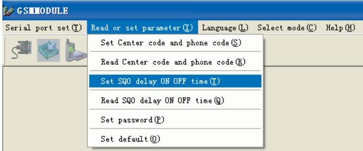
Input SQ0 Delay ON time Click “ Set Delay ON time ” and download Delay ON time to SMS module.
