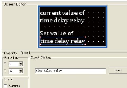
Choose the component “ **BE** ” , and select “ Function block B0003 (ON-delay).The “ current value ” is chosen as the parameter. Displayed digits: 2; decimal digits: 0
