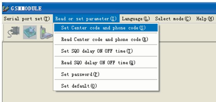
Input SMS center number and SMS mobile number. SMS center number is 20bits at most. It is the operating agencies message service center number of SIM card in SMS module, e.g.: 861380025500. " SMS mobile number " : 20 bits at most. If it is not set, no any message will be sent when there is the alarm.
