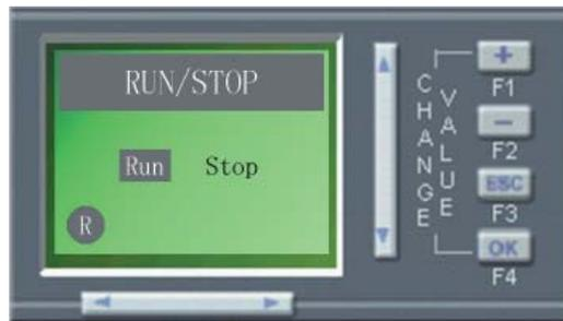
On this interface, change the cursor position by moving “  $\leftarrow \rightarrow$  ” key. Select “ Run ” or “ Stop ” and press “ OK ” key to confirm. Press ESC to return to the main interface.
