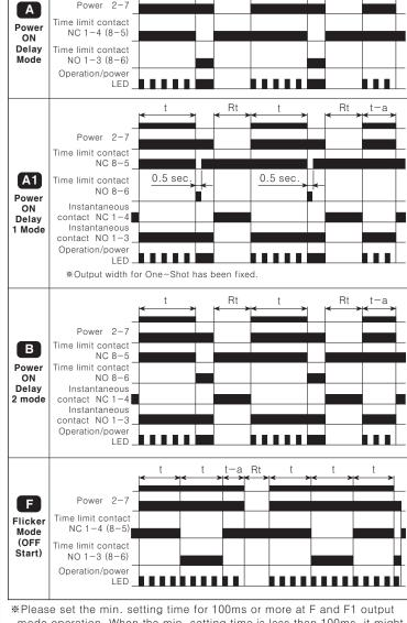
mode operation. When the min. setting time is less than 100ms, it might not be operating normally due to relay contact reaction time
