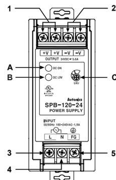
※SPB-015/060 Series has an output power [+V] terminal (1) and an output power [-V] terminal (2).
